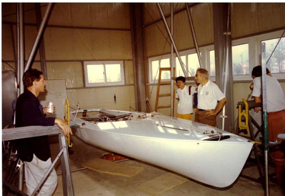
Figure H.4.8.2 A Flying Dutchman on a bifilar suspension at the 1988 Olympics in Pusan. Note the lightweight hooks and cross wire. The Lambolley hooks were used for subsequent pitch radius of gyration measurements for comparison.
