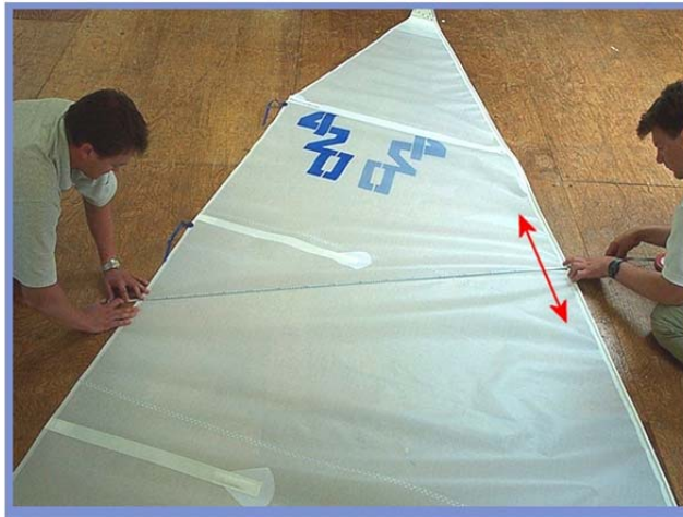
Figure K.2.3.8 Mainsail half width.
