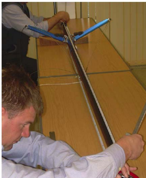
Upper point from MDP. Spar length measurements are to be taken along the spar (ERS H.4.1) so any curvature on the spar must be followed closely.
