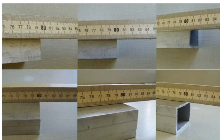
Figure F.4.3 The parallax error when sighting a non-contiguous scale
