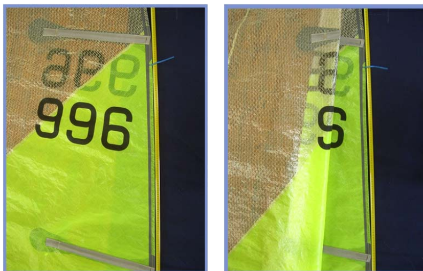
Figure K.2.3.3 Leech hollow before and after flaking.
