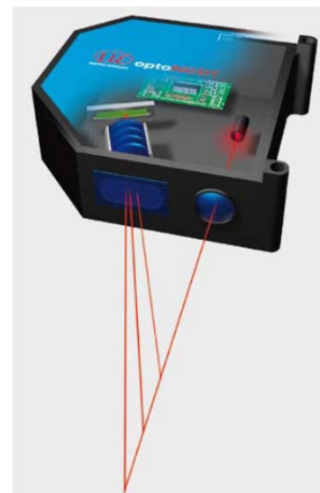
Figure F.6.2.2 A laser triangulation sensor
