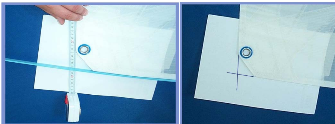
Figure K.2.1.2 Clew point marked on paper.
