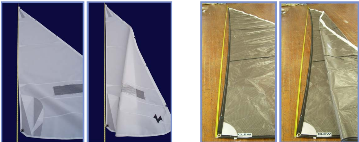
Figures K.2.3.1 & K.2.3.2 Leech flattening before and after flaking.
