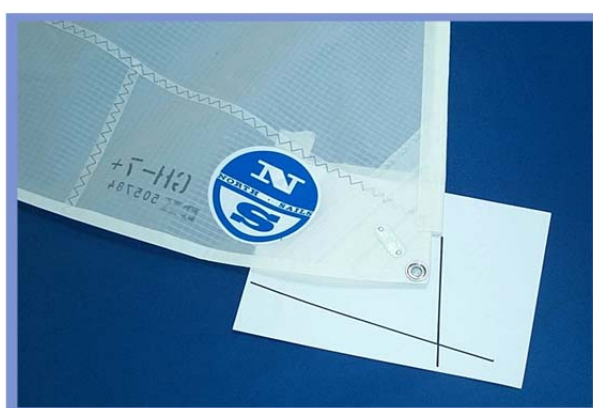
Figure K.2.1.3 Tack point marked on paper.
