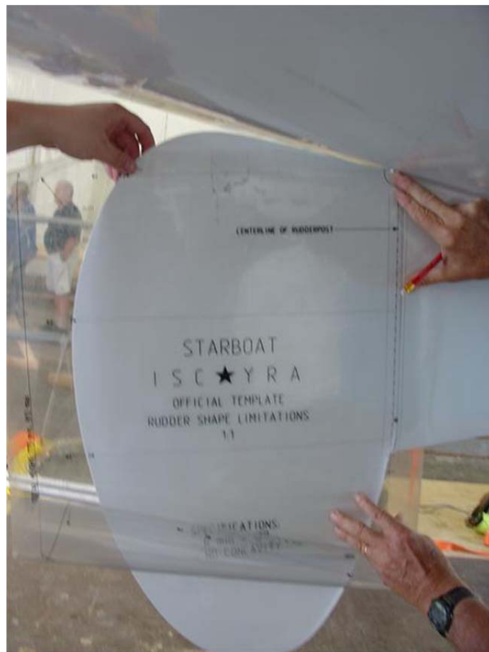
Figure I.5.4 Profile check with mylar template.
