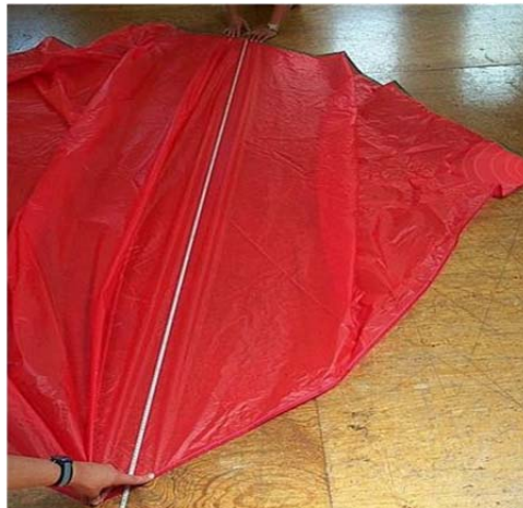
Figure K.2.3.10 Spinnaker half width.
