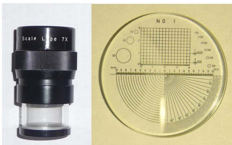
Figure K.1.2.5 An X7 Lupe with measuring reticule for sail cloth identification.
