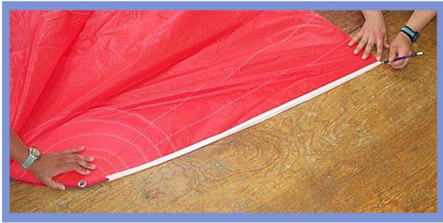
Figure K.2.2.3 Spinnaker mid foot point.
