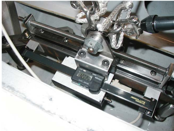
Figure H.4.7.2 The 2004 tilt swing system installed on the keel bolts of an Yngling. The swing bearing is mounted on a precision rail and the position read on the electronic scale. The box below the “rail scale” is the inclinometer. The roller bearing and the shackles for the support and steady lines of the suspension can be seen at the top of the photograph.
