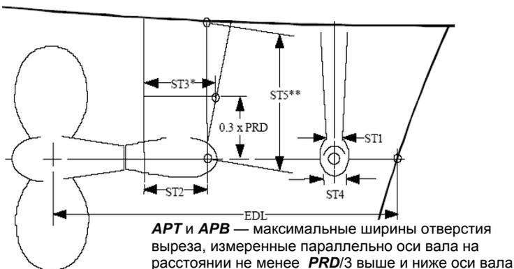
APT and APB are the maximum aperture measured parallel to the propeller shaft, found less than  $PRD/3$  above and below the shaft axis
